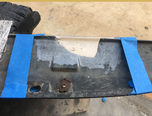
I used a bit of plastic as a backing...
