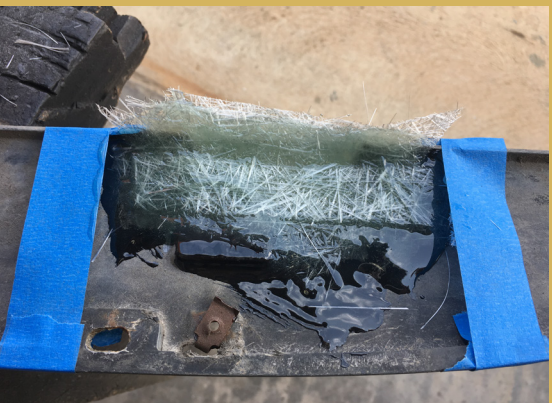
Use about 5 layers of fibreglass
