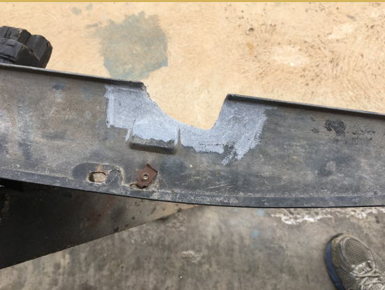
Grind away to create a wide chamfer
